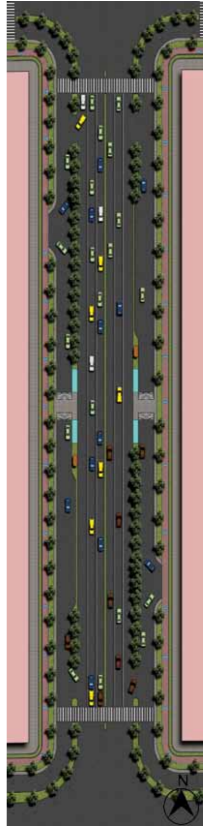
Typical view of the proposed side road showing the modified ROW from 10-12m (existing) to GOM with three lanes on the either direction.
